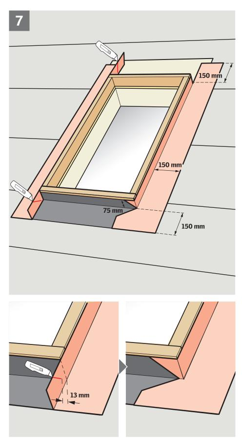
Consider wrapping the curb with VELUX adhesive skylight underlayment ZOZ 216 and create water-shedding laps over felt at bottom and sides of skylight **6**, **7**.
