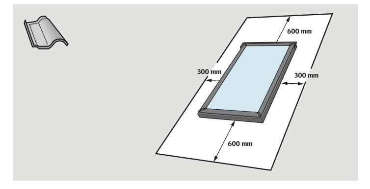
Maintain illustrated clearances between skylight frame and critical areas such as valleys, ridges, slope changes and roof-to-wallintersections.
