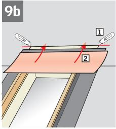
To allow for proper drainage, interweave felt with additional standard roofing underlayment as shown in a for new construction applications. For retrofit applications, interweave felt with additional standard roofing underlayment as shown in a.
