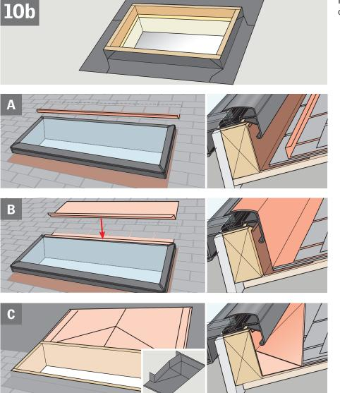
If custom-made flashing is used, consider options **A**, **B** or **C**.
