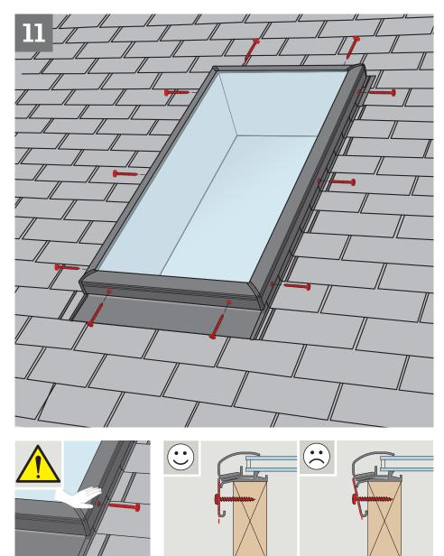
Centre the skylight on top of the curb and secure with 45 mm pan head stainless steel screws provided. Screws will penetrate the curb by at least 19 mm.
