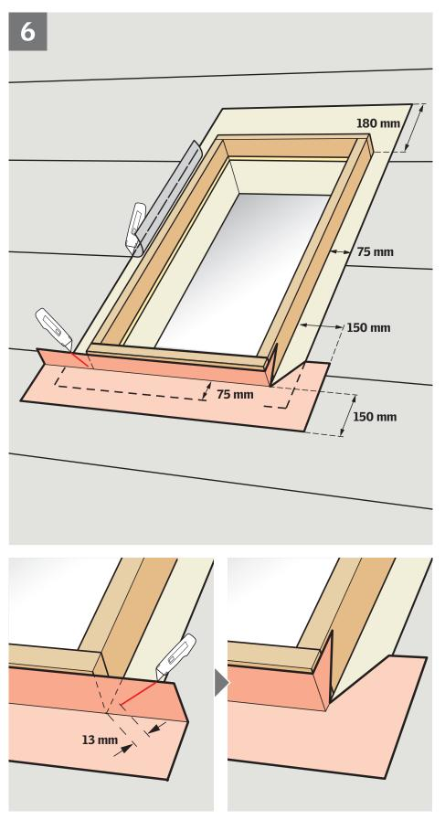
Skylight curbs should be completely wrapped in self-adhesive membrane to ensure waterproofing. To achieve this waterproofing, consider using VELUX adhesive skylight underlayment ZOZ 216 (225 mm wide).
