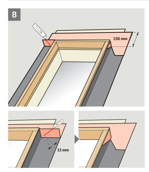
Consider wrapping the curb at top frame of skylight with VELUX adhesive skylight underlayment ZOZ 216 and create proper water-shedding lap.
